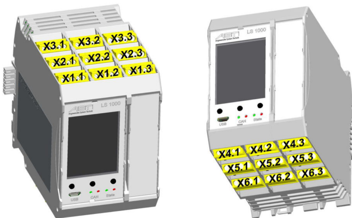
Figure 3 - Position of the connections LS 1104-B400-6/4-8
